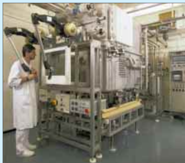
Fig. 4.12 – The stainless steel caisson for the pyro-processing installation at the Institute for Transuranium Elements, JRC Karlsruhe
