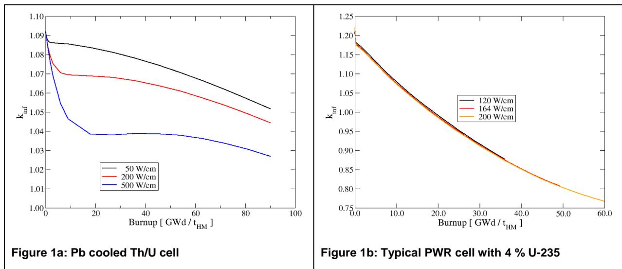
**Figure 1: Influence of linear power rate on criticality for different fuel and reactor systems during burnup**
