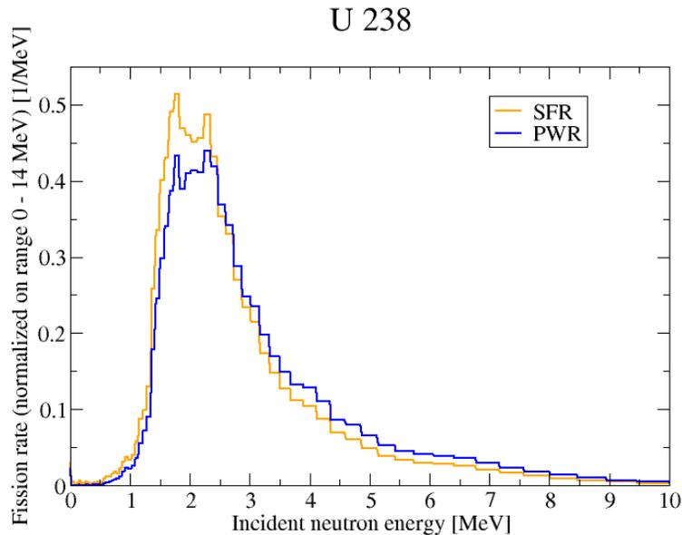
**Figure 2. Fission Reaction Rate of  $^{238}\text{U}$  per Unit Energy, Condensed on 10 keV Bins**
