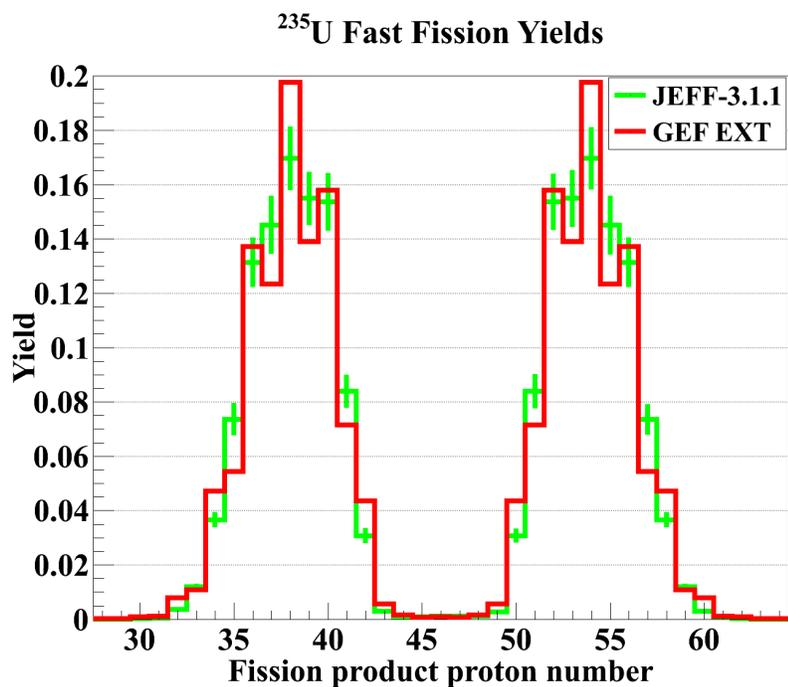
Figure 3. Calculated Fast Fission Yields of  $^{235}\text{U}$  vs. JEFF-3.1.1 Data
