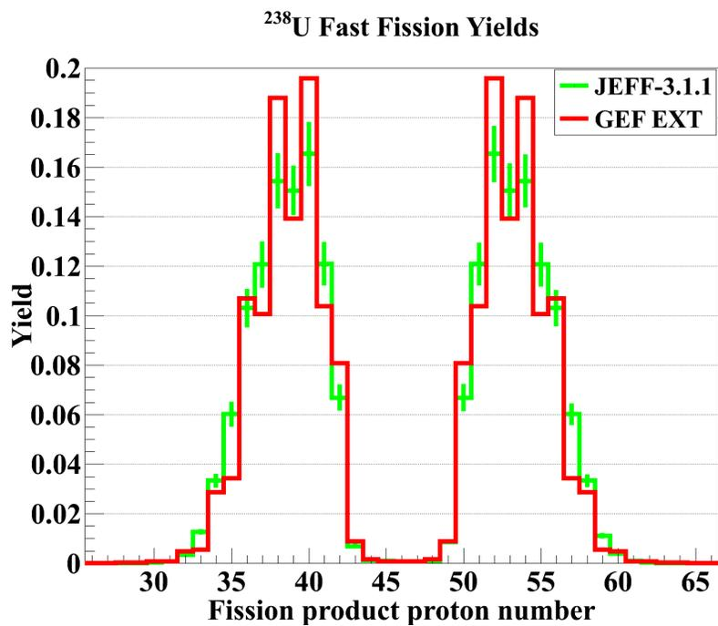
Figure 4. Calculated Fast Fission Yields of  $^{238}\text{U}$  vs. JEFF-3.1.1 Data
