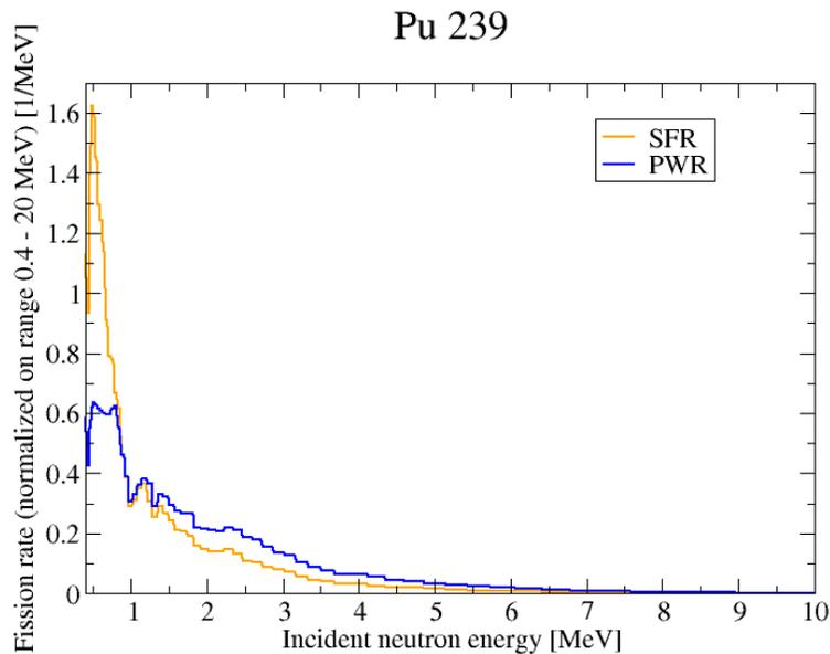
**Figure 1. Fission Reaction Rate of  $^{239}\text{Pu}$  per Unit Energy, Condensed on 10 keV Bins**
